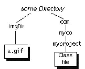
To create an Image object using the a.gif image file under imgDir, the applet can use the following code:
