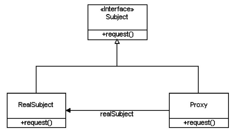
**RMI uses the Proxy design pattern.** The stub class plays the role of the proxy, and the remote service implementation class plays the role of the RealSubject. Skeleton is analogous class on the server side (obsolote until java 1.2).
