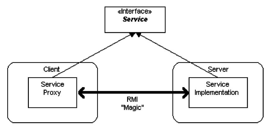
RMI supports two classes that implement the same interface. The first class is the implementation of the behavior, and it runs on the server. The second class acts as a proxy for the remote service and it runs on the client.
