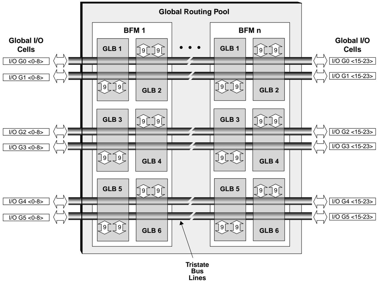
configured as an extension of an external tristate bus using the bidirectional capability of the I/O cells connected to the Global Routing Plane. The Global Routing Plane I/Os 0-8 and 15-23 from each group (I/O Gx as defined in the I/O Pin Location Table) can connect to the internal tristate bus as well as the unidirectional/non-tristate global routing channels. I/Os 9-14 connect only to the global routing channel.
