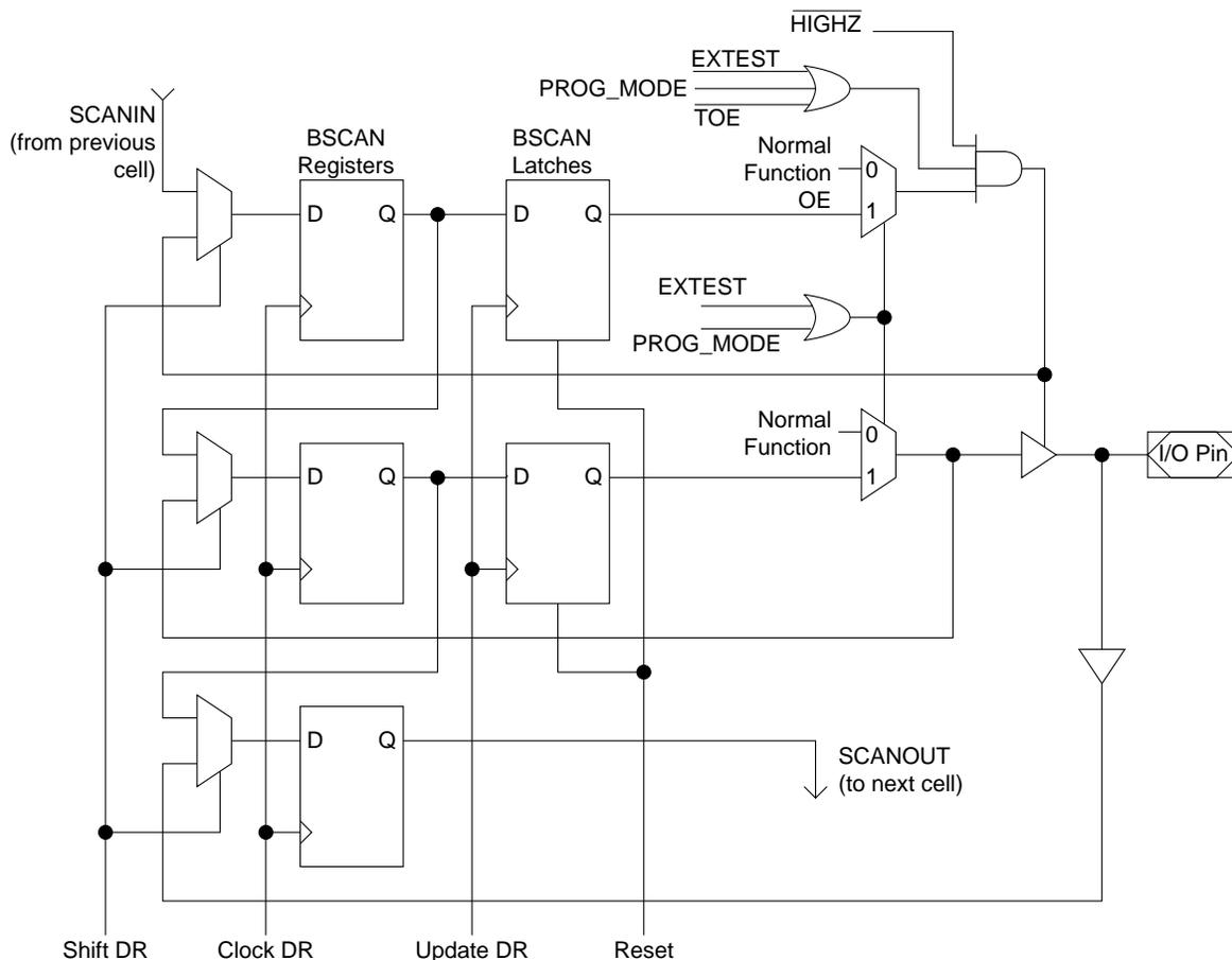
Figure 7. Boundary Scan Register for Dedicated Input Pins
