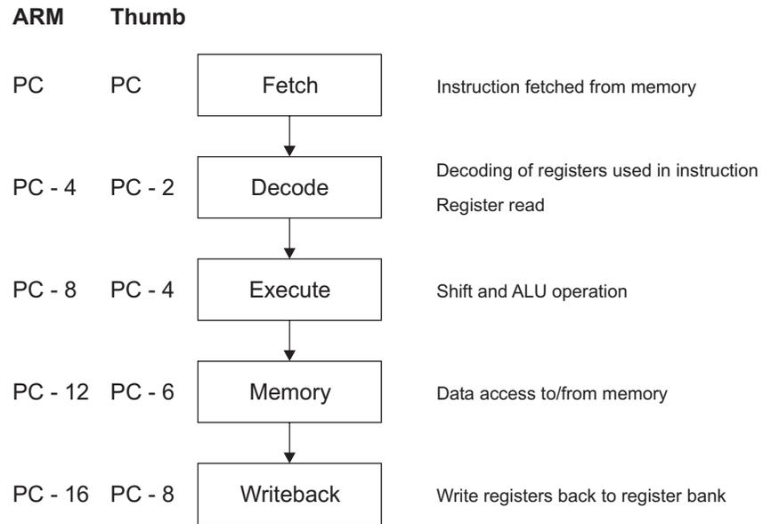
**Figure 1-1 Five-stage pipeline**
