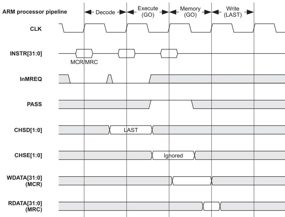
Figure 6-3 ARM9E-S MCR or MRC transfer timing
