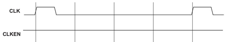
**Figure 5-2 Stopping CLK for power saving**
