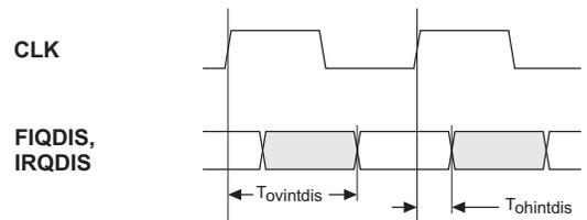
**Figure 9-7** Interrupt sensitivity status timing
