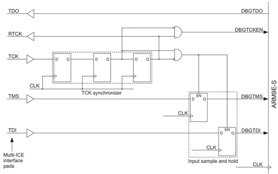
Figure 7-7 Clock synchronization
